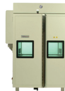
Qualmark 6-Axis HALT/HASS Chamber for GMN8020 Specification Including Intermittence Detection
