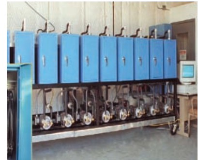
10-BAY & 5-BAY Fuel Recirculation Stands Multi-Temperature / Multi-Fuel Capability Temperature Range 50°F to 180°F (10°C to 82°C)
