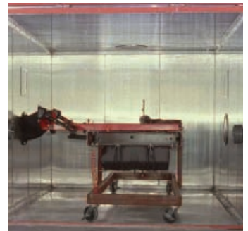
Vapor Recovery (ORVR) SHED Capable of Ambient Temperatures +55°F to 140°F (13°C to 60°C)
