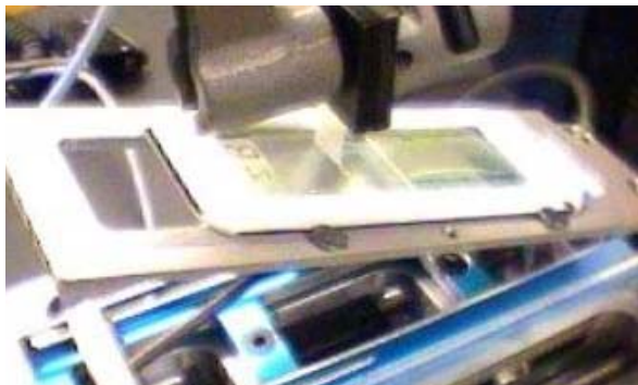
Measuring the interfacial work of adhesion for a polymer against glass.
